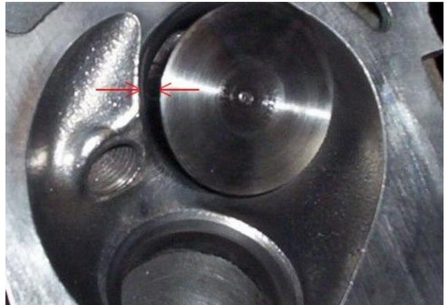
The valves themselves also need attention. There is a ridge in the back of each valve head, almost like a step. This needs to be considerably smoothed. Mounting the valve stem in the chuck of a drill and using emery paper on the valve head is an easy method of dealing with this.
