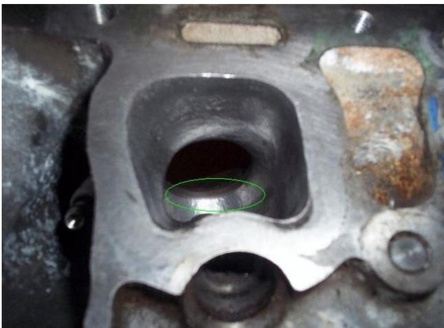
Valve seat step removed and valve seat blended into port walls
