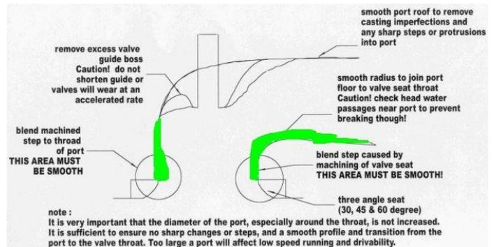
The biggest single area needing attention for both inlet and exhaust valves is the step left in the casting of the cylinder head by machining to fit the valve seat inserts. This can be seen in the following picture, circled in green:
