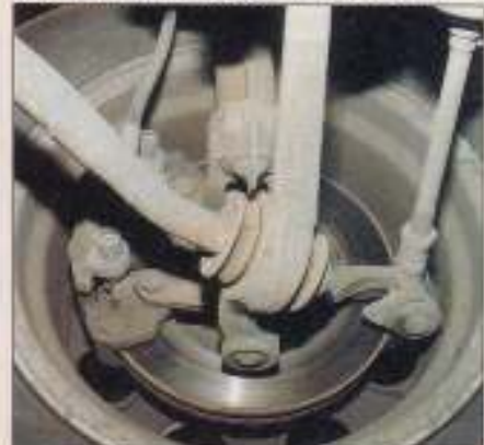
Front suspension and steering require close scrutiny, especially the multitude of rubber bushes, brake discs (they often wear rapidly), and the steering rack (watch for torn gaiters).
