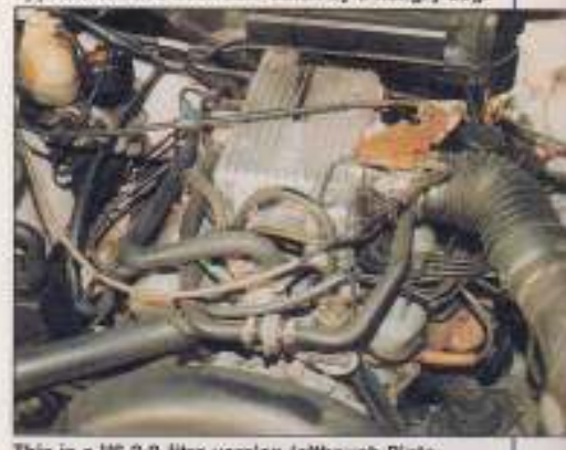
This is a V6 2.8-litre version (although Pinto powered Sierras predominate). Check for oil leaks, 'top end' noise and timing gear rattle. On Pinto units, watch for oil leaks and smoking, and listen for clattering from worn camshaft/followers.
