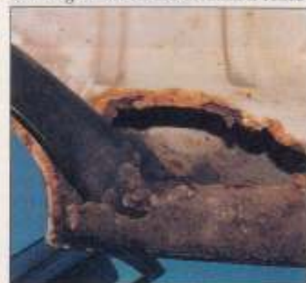
Don't be deceived by a bonnet which looks good from outside. Open it and view the underside of the assembly from below. The leading edge collects moisture and salt, then holes appear.
